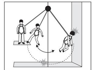
We will ensure as far as it can to focus on work situations with a fall factor 0 or 1 and we will be avoided if possible to install a fall arrest system on an anchor in fall factor 2, the pendulum effect must also be as small as possible.
